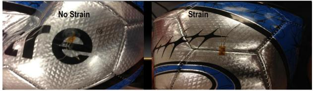
stitching of the soccer ball when completely deflated, and voltage differences were measured across two nodes on a Wheatstone bridge for 4 psi, 7 psi, and 10 psi. The experiment showed that the used ball deformed more with increasing internal air pressure than the new ball.
